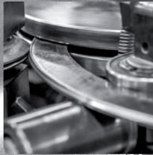
Fabrication de joint spirale Spiral wound gasket manufacturing
